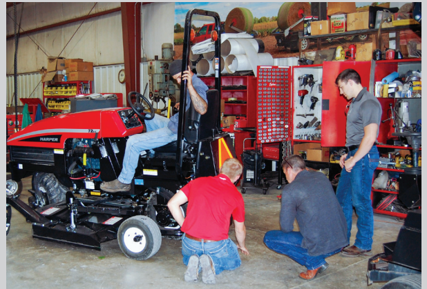
Left: Logan Livengood inspects a TV35, a self-contained turf vacuum that verti-cuts and vacuums all in one pass.
